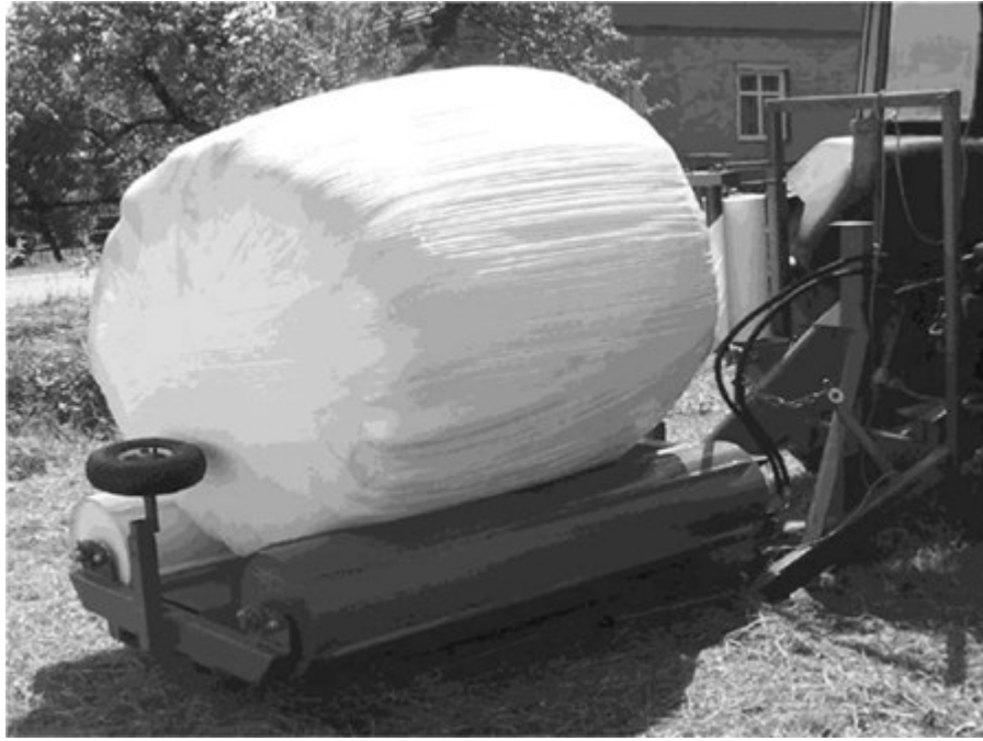
Fig.6 Bale after the end of the wrapping
