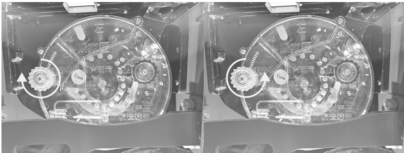
Increase seed quantity released to chamber.
