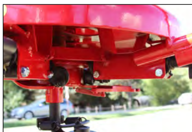
Spheroidal cast iron cam and steel rollers.
