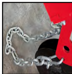
Heavy chain to ensure seed coverage
