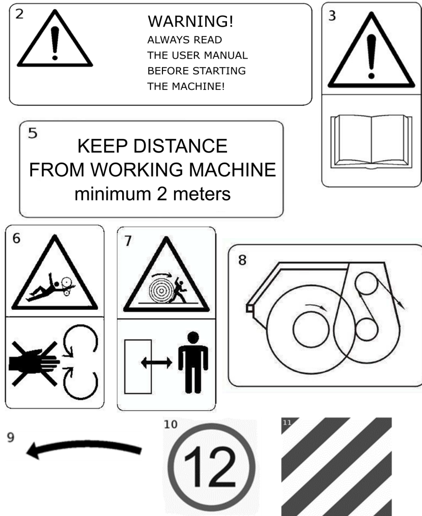
Fig.3 Safety stickers and information plates – explanation:
