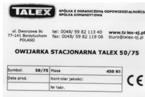
Fig.5 Identification plate - pattern
