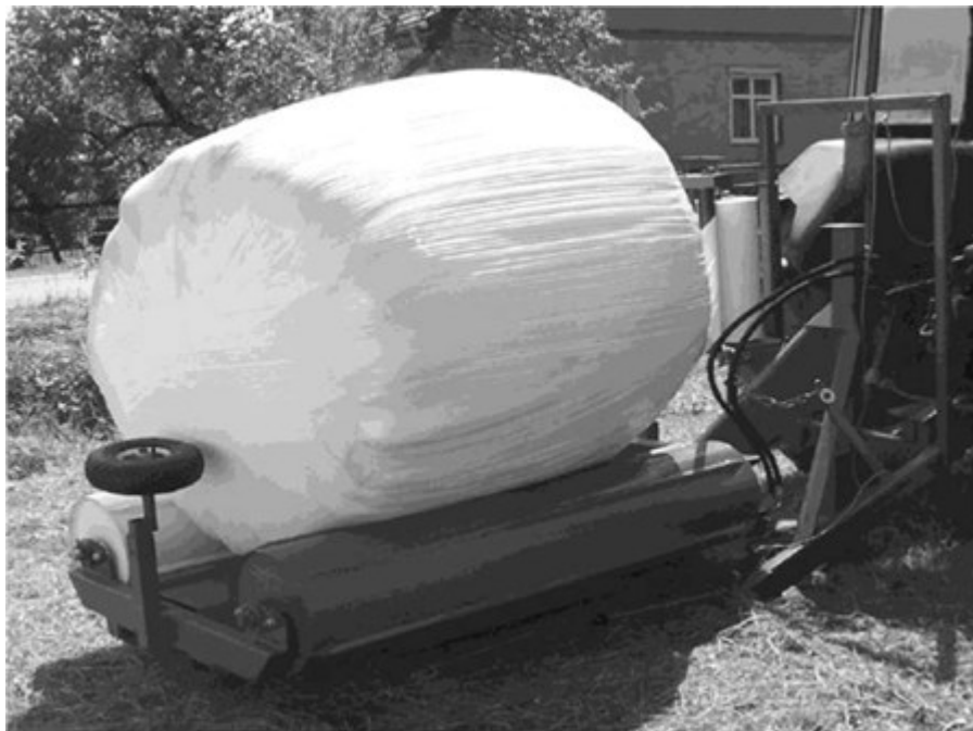
Fig.6 Bale after the end of the wrapping
