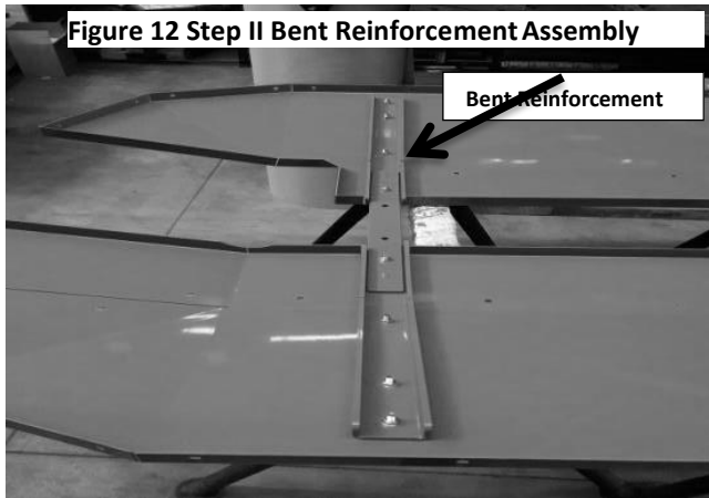
Figure 13 Step II Bent Reinforcement Assembly
