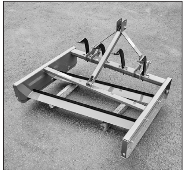
Figure 4: Land Grader blocked up on 4" x 4" wooden supports.
