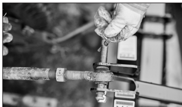
Install center link and mounting hardware.
