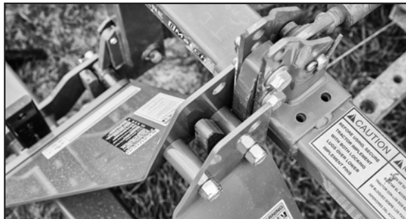
Raise quick hitch and engage hitch pins.
