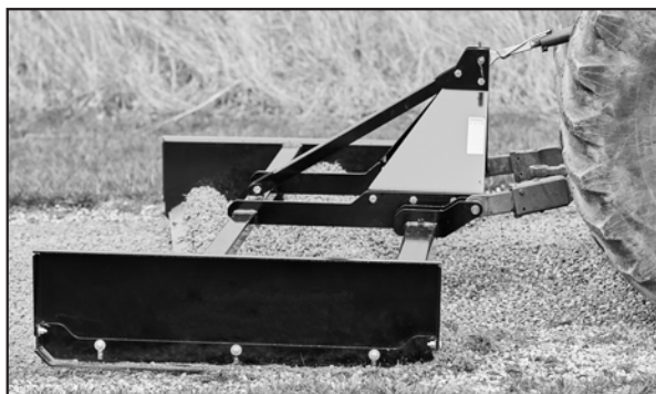
Ensure implement is level when lowered to the ground. NOTE: Scarifier shanks not shown.
