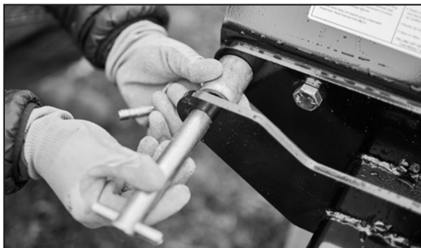
Install bushings before attaching to quick hitch.
