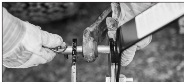
Attach tractor draft link to hitch pin.
