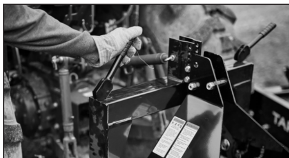
Lower handles to lock quick hitch.
