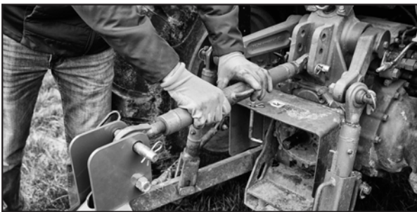
Figure 2: Use tractor top link to tilt front and rear of Land Grader.
