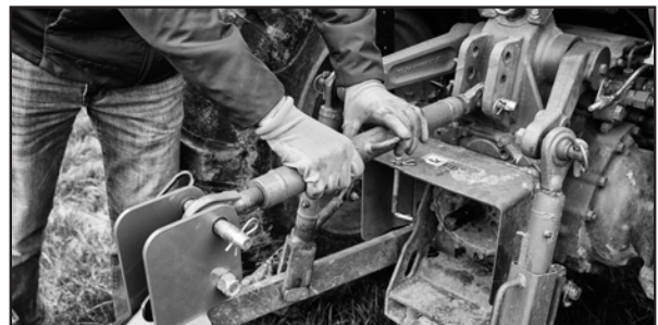
Figure 4: Use tractor top link to tilt front and rear of Box Blade.
