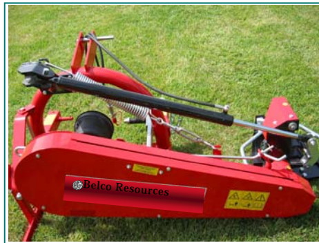
Hydraulic lift standard on most sizes
